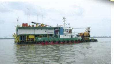
The offshore pipelines are laid with accuracy of  $\pm 5$  m while the platform position is fixed. A comprehensive metrology is performed by divers to finalize the length of the dogleg based on the actual position of the laid pipeline. The dogleg spool is fabricated on the barge itself. The final tie-in is done in 2G position at the location above the riser clamp.
